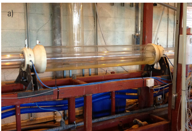
a) Displacement results were obtained using a 10 m long flow loop with distributed conductivity probes for detecting the fluid interface position during displacement. b) Numerical simulations using a 3D open-source platform have been performed to analyse the experiments.
